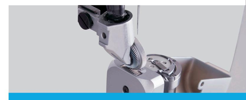
Full Automatic Drive Roller Slim Post Bed Sewing Machine With Top And Bottom Feed
